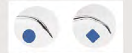
Figure 4: Ultrasonic Instrument Cross Section. Figure 4a round/cylindrical cross section absent of rounded corners. Figure 4b square/rectangular cross section with rounded corners.
